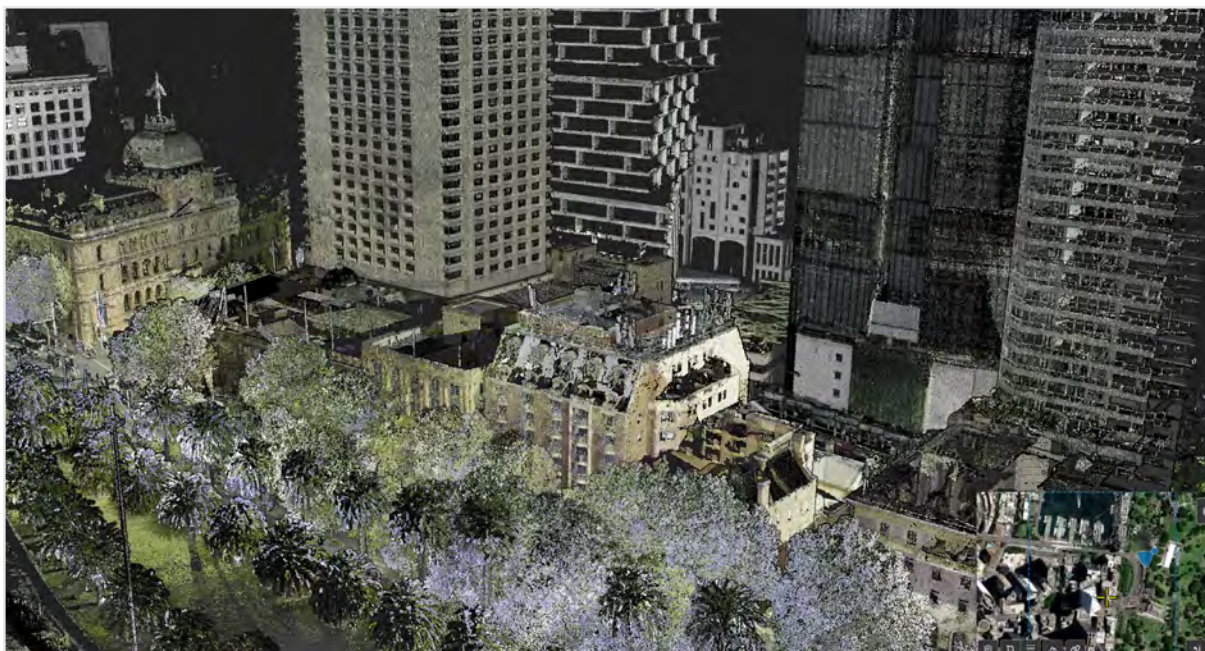
Figure 5a – LEICA Point cloud survey provided by CMS Surveyors
